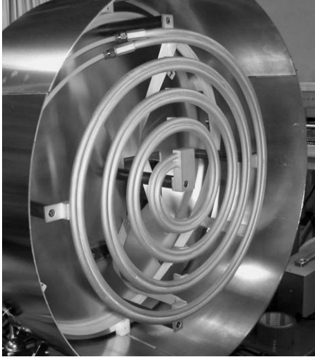
Fig. 3. Large diameter (43 cm o.d.) spiral antenna.
